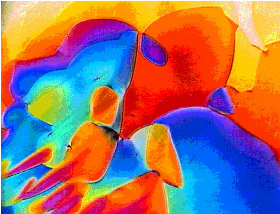
Figure 4. Texture of the TGBA* phase in a cell of gap d = 8 \mu\text{m} with planar boundary conditions. The molecular long axes are oriented in the plane of the substrate, and the helix axis is perpendicular to the bounding glass plates. The photograph was taken on cooling the sample; different colours correspond to different twist states due to hysteresis effects and a non-uniform temperature distribution.
